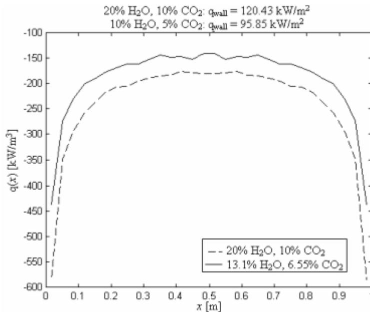
Figure 3. Volumetric radiative heat rate and heat flux on the walls for gas mixtures having concentrations of 20% H<sub>2</sub>O and 10% CO<sub>2</sub> and of 13.1% H<sub>2</sub>O and 6.55% CO<sub>2</sub>. Gas mixtures temperatures of 1780 K.
