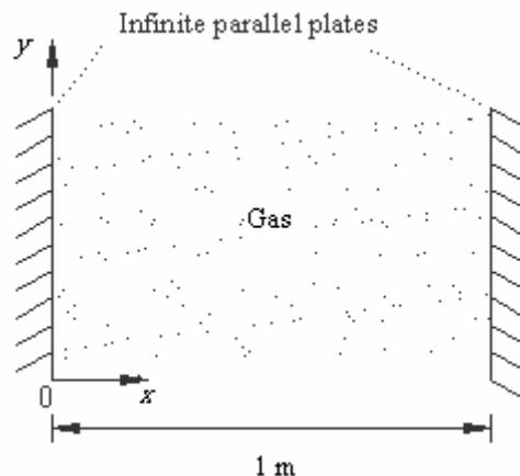
Figure 1. Gas layer between infinite parallel walls.
