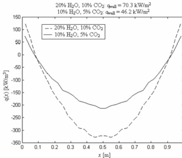
Figure 5. Volumetric radiative heat rate and heat flux on the walls for gas mixture having concentrations of 20% H<sub>2</sub>O and 10% CO<sub>2</sub> and of 10% H<sub>2</sub>O and 5% CO<sub>2</sub>. The gas mixtures temperatures are given by Eq. (17).
