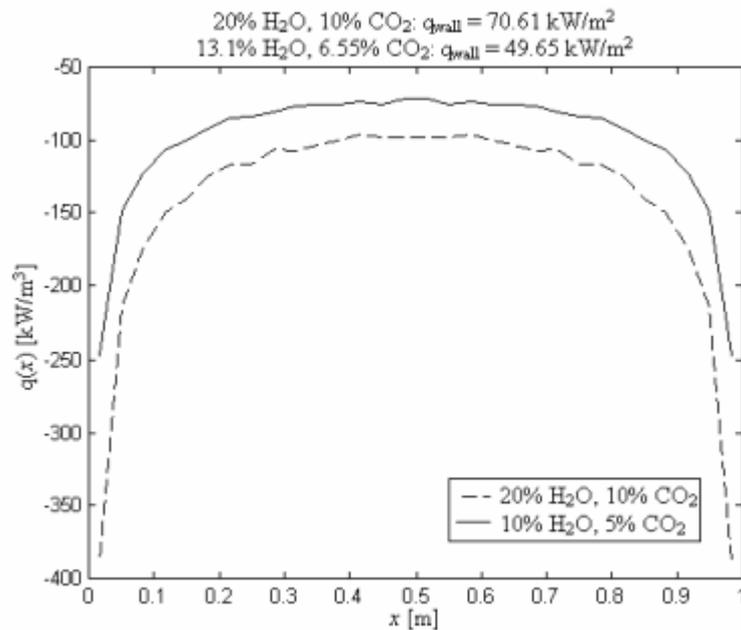
Figure 4. Volumetric radiative heat rate and heat flux on the walls for gas mixtures having concentrations of 10% H<sub>2</sub>O and 10% CO<sub>2</sub> and of 10% H<sub>2</sub>O and 5% CO<sub>2</sub>. Gas mixtures temperatures of 1476 K.
